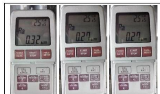
Figure 12. 1400 rpm Surface Roughness
