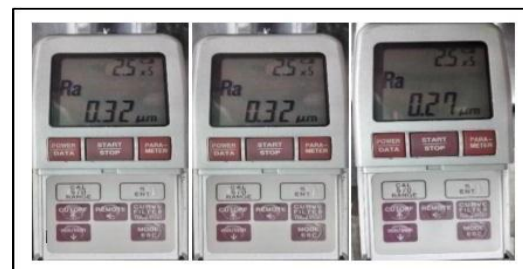
Figure 11. 1200 rpm Surface Roughness
